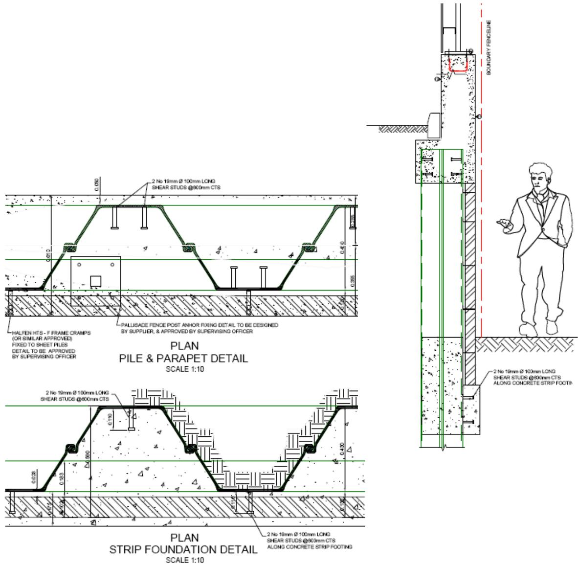
**Figure 1:** Example of original proposed sheet piled wall with brick cladding design
