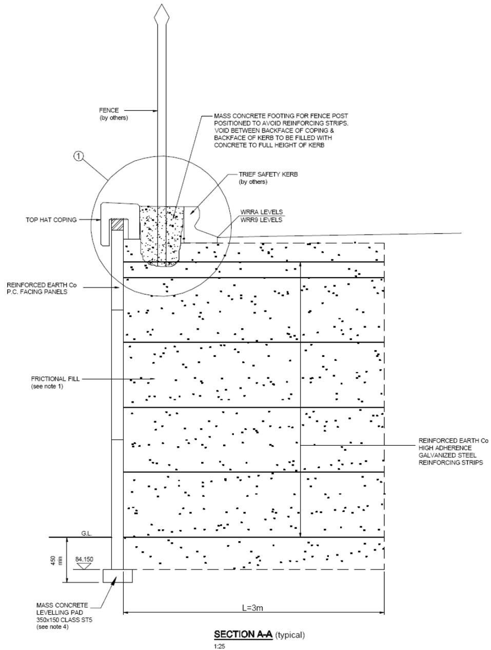
**Figure 2:** Example of Concrete Panel Wall with steel strips reinforcement used at Hunters Lane
