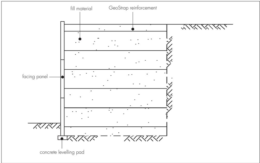
Figure 7 Typical reinforced soil structure — diagrammatic plan view
