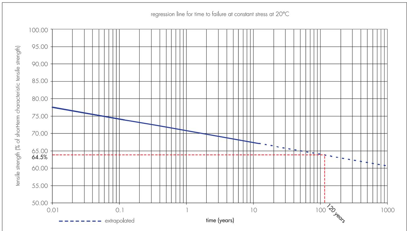
7.4 For a 120-year design life and design temperature of 20°C, the long-term tensile strength ( $T_{CR}$ ) for GeoStrap Reinforcement can be taken as 64.5% of characteristic short-term tensile strength ( $T_{char}$ ), giving a long-term creep reduction factor ( $RF_{CR}$ ) of 1.55.
