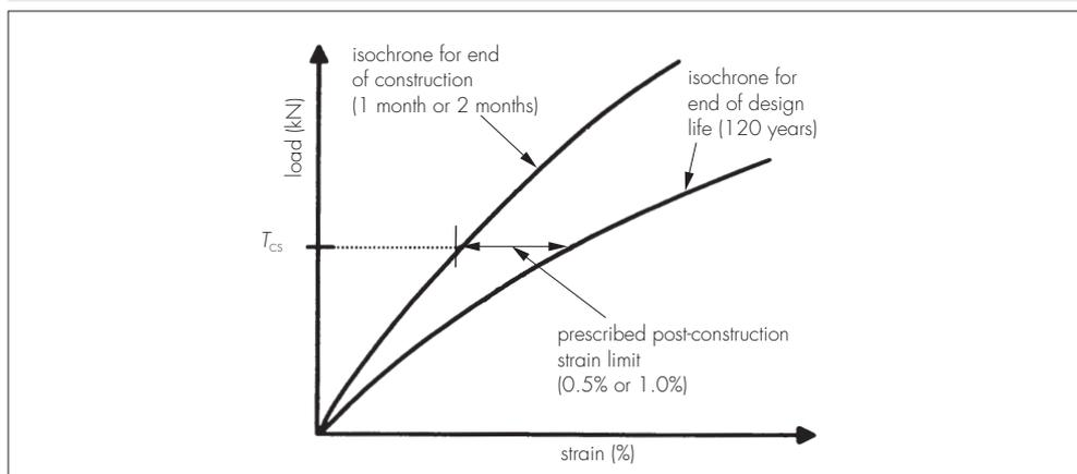
7.7 Reduction factors  $RF_{CR(SLS)}$  for determining  $T_{CS}$  from the characteristic short-term tensile load ( $T_{Char}$ ) for each grade of GeoStrap Reinforcement are given in Table 3. The following formula is used to calculate  $T_{CS}$ :
