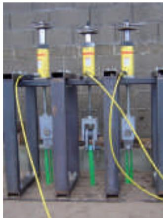
*Strength testing the panels under the effect of the tensile load of reinforcements*
